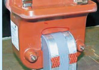
Deterioration of epoxy resin due to long-term use, resulting in cracking
