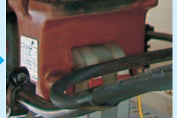
Cracking develops and causes partial discharge, resulting in a grounding fault
