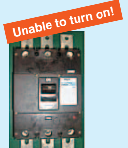
Unable to turn on again after a trip, making the breaker not work
